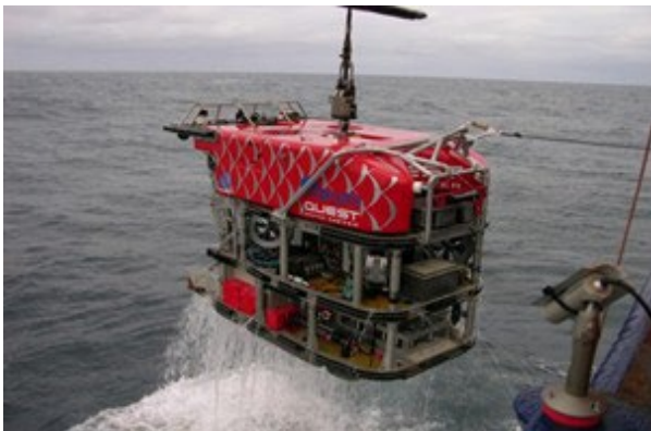
Quest 4000 ROV for deep-sea exploration. Photo: NOAA
